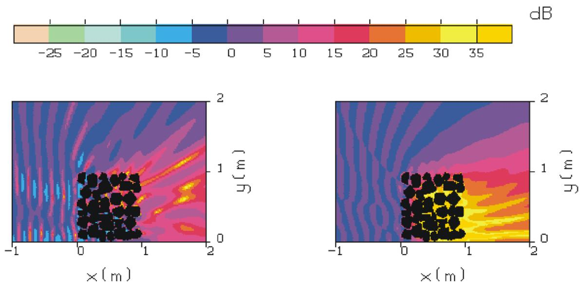
Figure 4. Insertion loss at 1000 Hz near a 1-m high and 1-m wide gabion barrier placed on rigid ground. On the left, rigid stones have been considered, on the right the equivalent case with expanded clay stones (flow resistivity of  $82 \text{ kPas/m}^2$ ) is depicted (From Ref. [49]).
