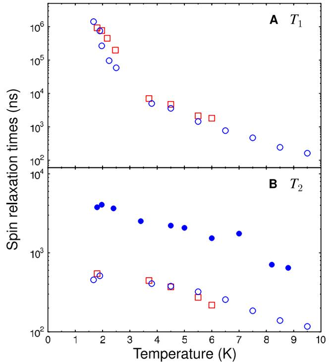
FIG. 3 (color online). (a)  $T_1$  as a function of temperature in  $\text{Cr}_7\text{Ni}$  (blue open circles) and  $\text{Cr}_7\text{Mn}$  (red open squares). (b)  $T_2$  as a function of temperature for  $\text{Cr}_7\text{Ni}$  (blue open circles),  $\text{Cr}_7\text{Mn}$  (red open squares), and perdeuterated  $\text{Cr}_7\text{Ni}$  (blue filled circles).
