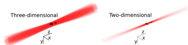
Fig. 7. Diagram showing how a collection of spherical scatterers in a three-dimensional beam (left) can be approximated in a two-dimensional system (right) where fields and scatterers extend uniformly in the  $y$  direction. The scatterers are, thus, cylinders, depicted as circles in the  $xz$  plane.
